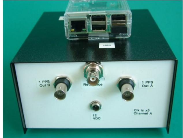
Figure 6. Rear Panel of TADD/TICC Enclosure
