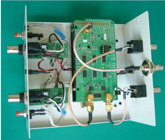
Figure 5. Interior of TADD/TICC Assembly
