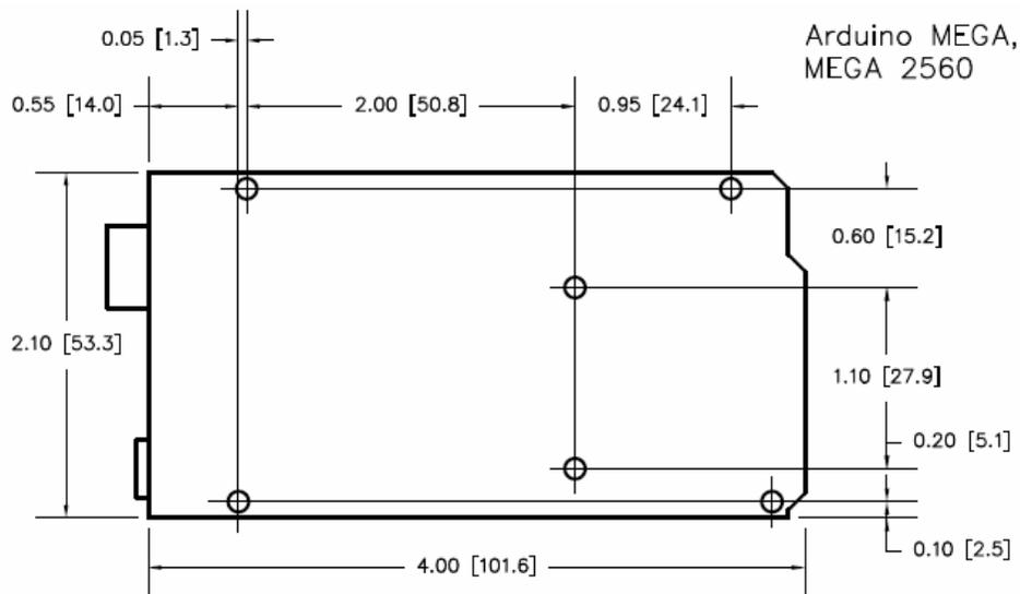
Figure 3. Arduino Mega 2560 Mounting Dimensions
